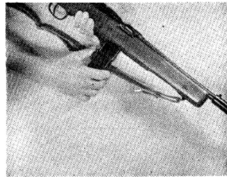
3. To Insert Magazine: Push up into Magazine Guide until Magazine Catch locks Magazine.
