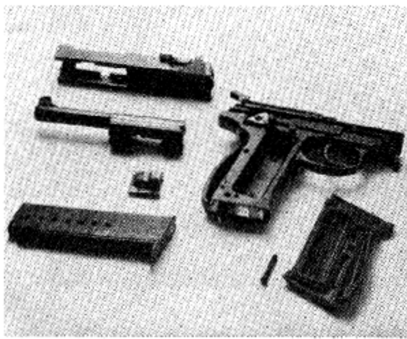
Top to bottom, left: Slide, barrel, lock, magazine. Top to bottom, right: Receiver, stock.
